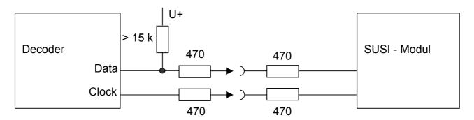
The decoder always acts as master and supplies the clock pulses. The first bit transferred is the LSB (bit 0).
